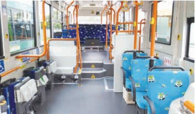
*Non-step buses have floors only 30cm higher than the road, making it easy for anyone to get on or off the bus.
