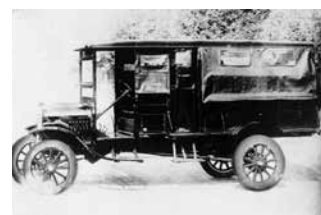
Entaro bus begins operation Model TT Ford 11-person conductorless bus (1924)
